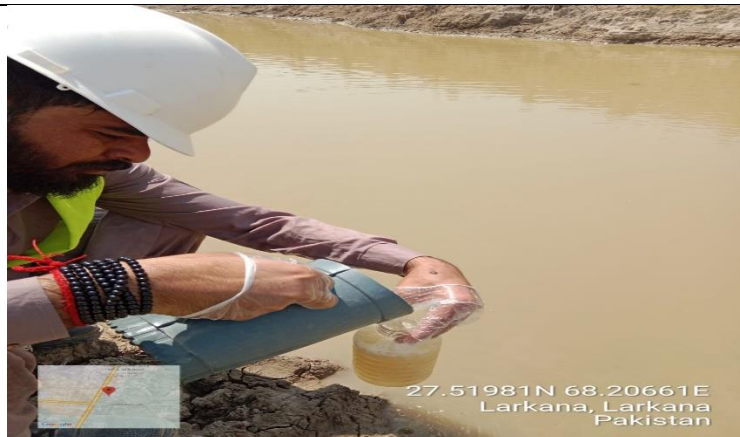
Surface Water Sampling
