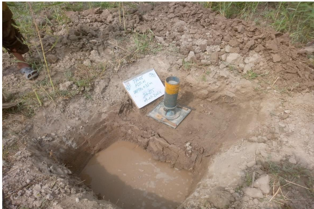
Photo-4: Performance of Field Density Test at TP-05.
