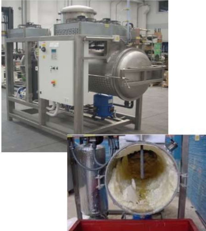
Figure 6.3: Brine Treatment System
