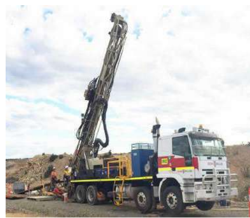
Seismic Drilling Rig
