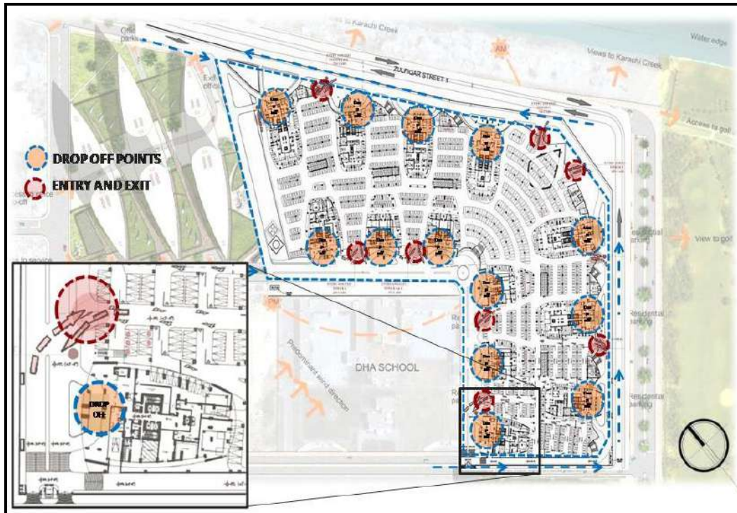
Fig 2.22: Internal Traffic Flow Plan for Residential Towers
